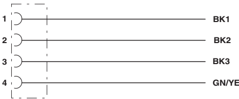
Contact assignment of the M12 socket
